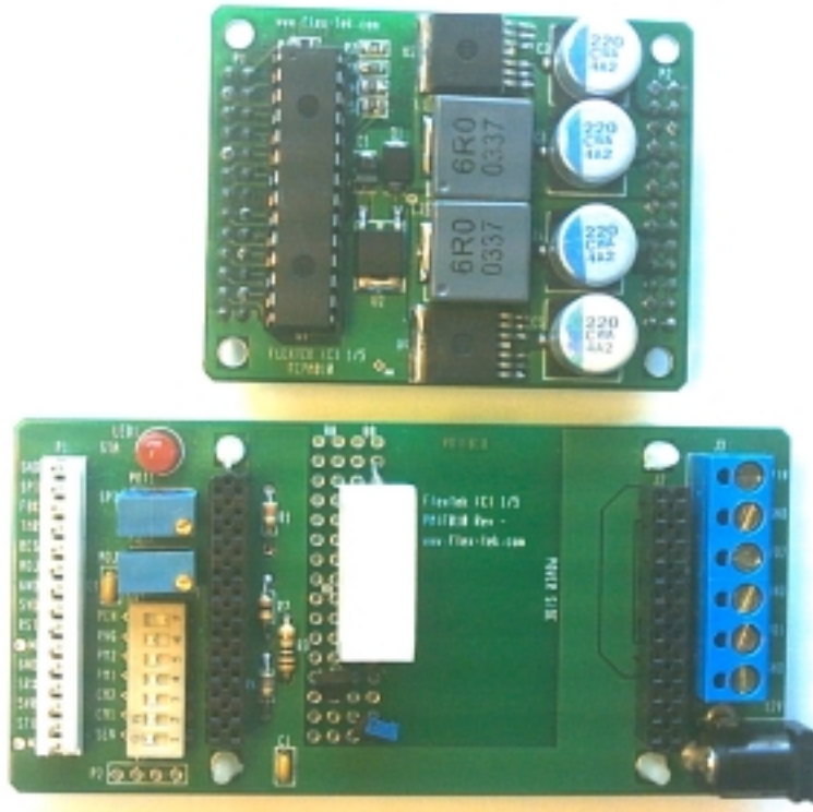
Figure 2. FlexConverter™ Evaluation Kit Photo (Compact Power Module Plugs into Evaluation Board for Convenient Operation)
