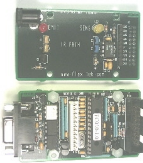
Figure 2.1. Education Kit Interface and Infrared Boards
